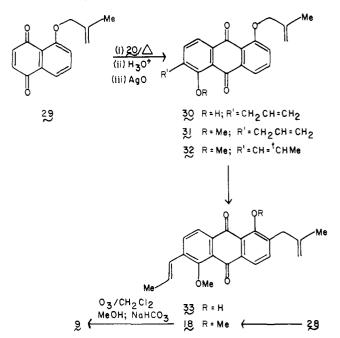
This crude product, which was in turn presumed to consist largely of 2-allyl-5-(methallyloxy)-1,9,10-anthracenetriol was oxidized with silver oxide to afford anthraquinone 30 which, upon methylation (73% overall), provided the methyl ether 31.
